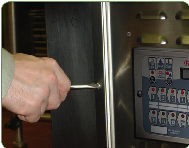
10. Plug the VC-210 harness connectors into the header assembly and secure to the header using the 2 screws provided on the controller.
