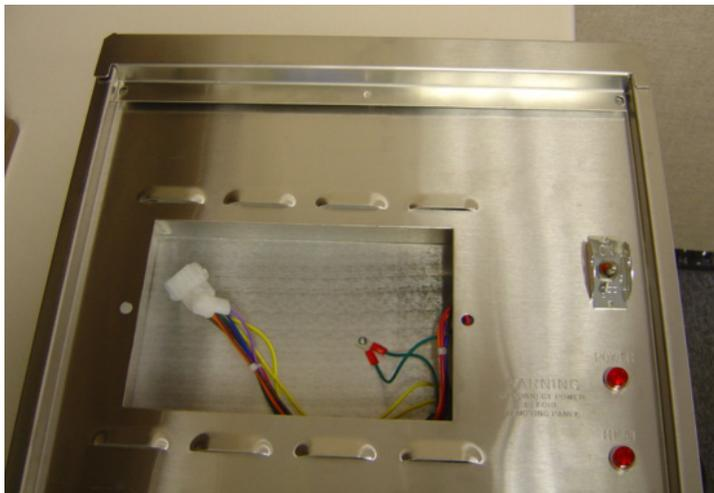
2. Using the enclosed hardware package, (part #213-50429-01), install the nut to stud and tighten.
