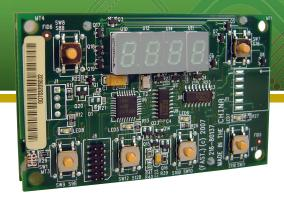
Multi-Parameter, Single Display, Multi-Function. Reliable and precise mid-level cook time and temperature control with easy-to-read display and 4 programmable product buttons.
