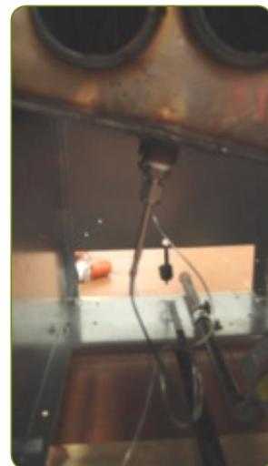
**4G:** Inside the vat verify the probe is positioned correctly. The length going down to the bottom of the vat is not touching the heat tube. The probe tip sticks out of the bracket about 1 in. Then on the bottom, tighten the compression fitting cap tightly.
