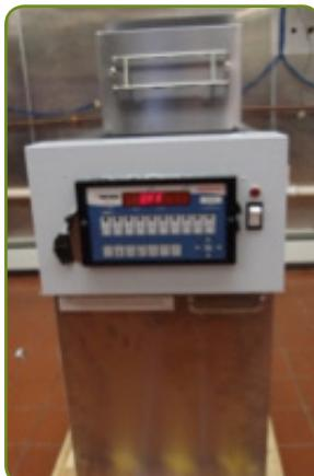
**11D:** Turn header power switch on. The indicator lamp should cycle on and off. Verify it cycles on and off a few times.
