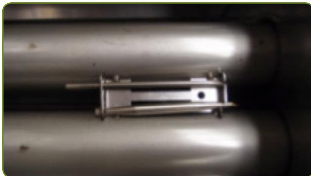
**4A:** Following the path of the original probe feed the ends of the probe wires down and through the probe hole in the bottom of the vat. It may be helpful to feed a stiff wire up from the bottom through the probe hole. Tie the probe wires to the stiff wire and pull the wires down through.
